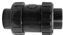
Rückschlagventil S4 DN80 PVC grau PVC-U Klebemuffe d110 metrisch PN6 EPDM EPDM Cone Check Valve S4 DN80 PVC grey PVC-U solvent socket ends d110 metric PN6 EPDM EPDM
